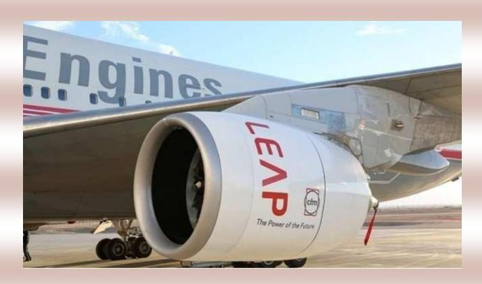
CFM International introduced their LEAP engine intended to compete with Pratt & Whitney PW1000 engine. This engine basically makes use of advanced material composites and different cool air mixing cycles modulating the amount of air flow to the internal passages inside its high pressure turbine to keep the temperature under control. The fan used in the engine has flexible blades manufactured by a resin transfer molding process, which are deigned to untwist as the fans rotational speed increases.
