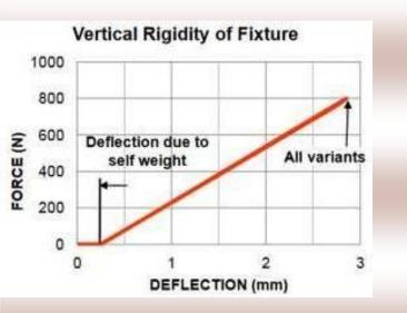
Look at the graphic above. At first the deflection is quite small due to door's self weight. However this deflection become larger when excessive vertical load is applied. Check the elasticity restoration when load is removed and make sure permanent deformation
