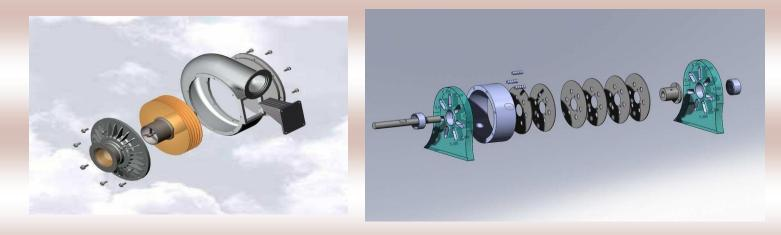
**CONSTRUCTION AND WORKING:** The Tesla turbine consists of a number of discs mounted parallel to each other on a shaft. Nozzles are located at the periphery of cylindrical casing and tangential to the shaft, pointing toward the inside. The discs are separated by thin gaps for the fluid to pass through it. Exhaust ports are located near the center of the turbine.
