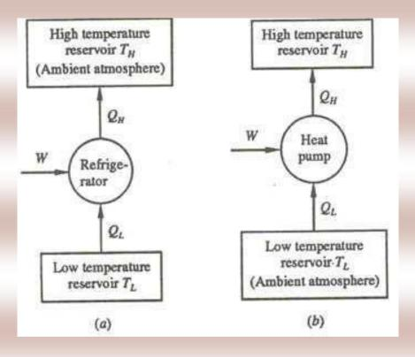
In general, the term heat pump is used to describe the cycle as heat energy is removed from the low-temperature space and rejected to the high-temperature space.
